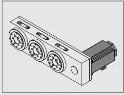
CNC .../Z... (2 to 5 spindles) multi-spindle 1-axis version
