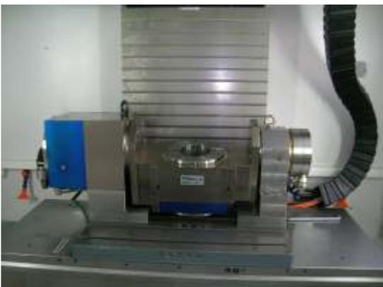
machine type: CINCINNATI CFVi 550 - 30 Tools (vertical machining centre)
