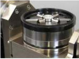
**Pallet clamping-systems** (manual or automatic):
